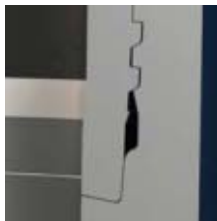
Toroidal seal makes sealability stable under any load case
